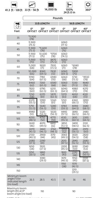
1.All capacities above the bold line are based on structural strength of boom extension and do not exceed 85% of tipping loads, in accordance with SAE J-765.
