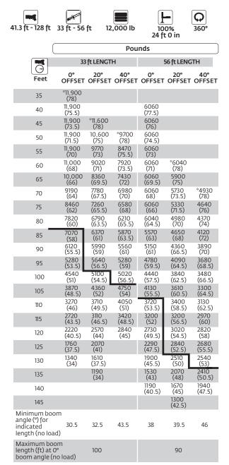
NOTE: ( ) Boom angles are in degrees. A6-829-103773 #LMI operating code. Refer to LMI manual for operating instructions. \*This capacity is based upon maximum boom angle.
