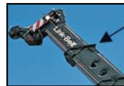
A-max extends only the inner-mid section of the boom for substantially increased capacities for in-close, maximum capacity lifts.
