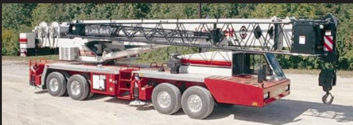
**Stowable Attachments** Swing-away lattice flies are easily stored for transportability or can be removed to meet specific road laws.
