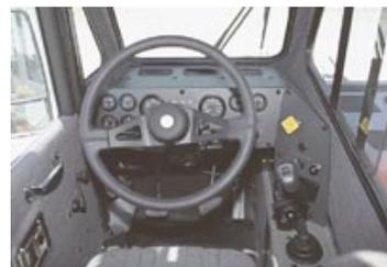
Additional features include dash mounted comprehensive instrumentation with attractive lighted gauges, sliding side and rear windows and roll up/down door window for excellent ventilation, fully adjustable air ride fabric seat, suspended pedals, and rear view mirrors. Cruise control and engine brake controls are conveniently located on transmission shift lever.
