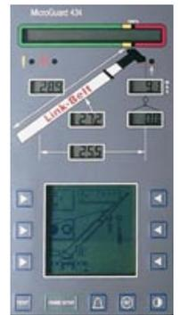
An exclusive new feature available on the HTC-8650 is the Operator Defined Area Alarm. By setting two points, the operator creates an imaginary vertical plane to maintain a safe working distance from nearby obstacles. Should the operator attempt to operate the crane beyond the plane, the RCL will sound an alarm.
