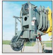
The RT700E has a quick-reeve boom nose and swingaway alignment device to help operators set up smoothly.
